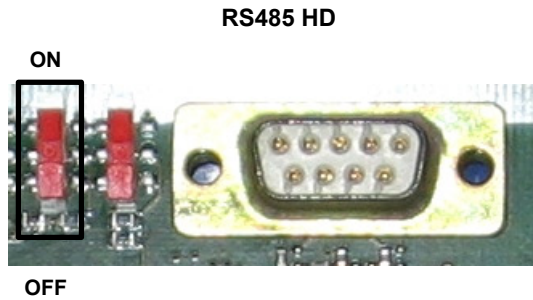
Figure 11 – RS485 HD Termination Resistance Switch
