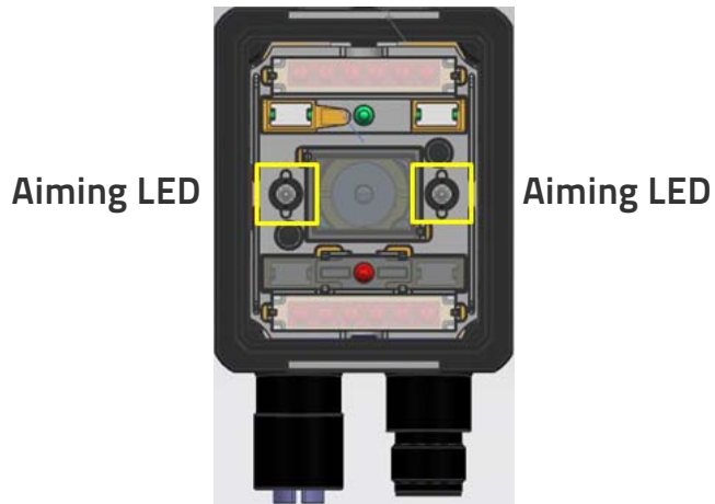
Figure 7 - Smart-VS Aiming LEDs
