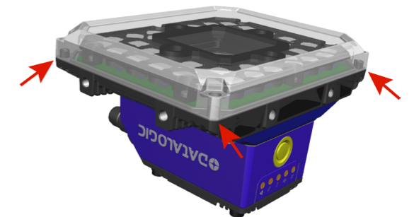
Fig. 2 - Removing the cover (36 LEDs model)
