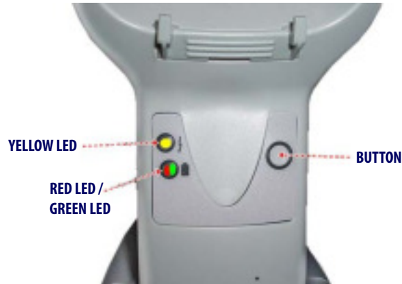
Figure 1. Gryphon I Base LEDs
